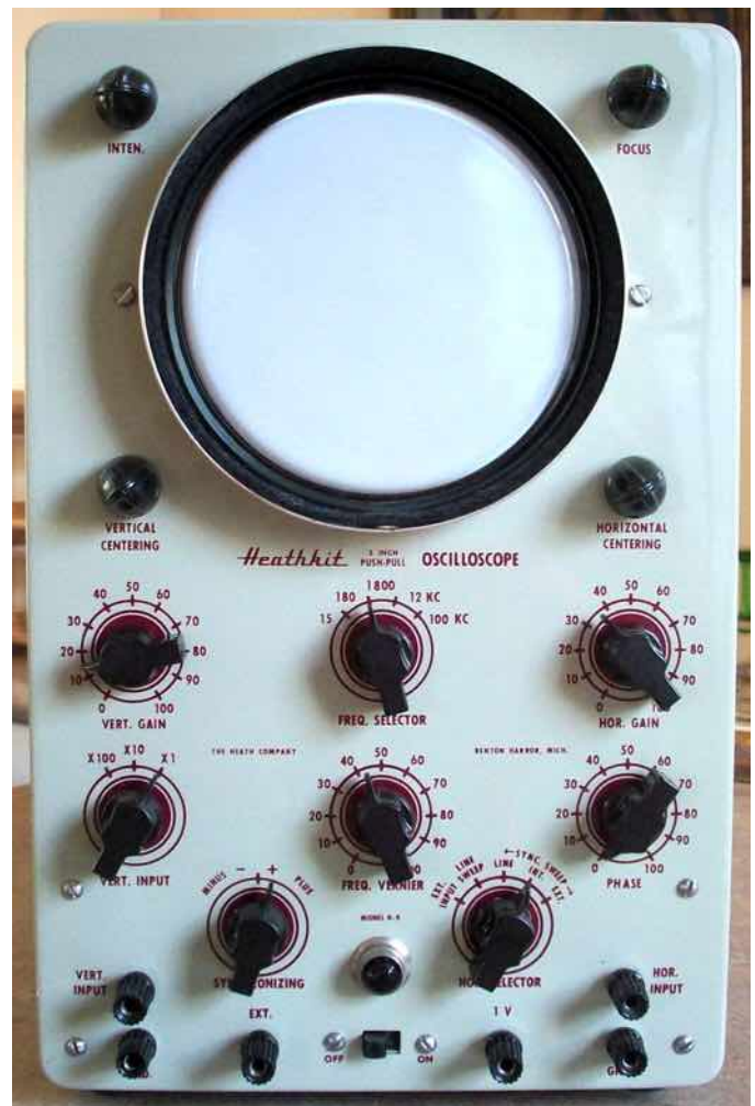
Figure 2: Heathkit O-9 Oscilloscope; last of the Late Pre-Classic style scopes. Photo by Keith Greenhalgh.
