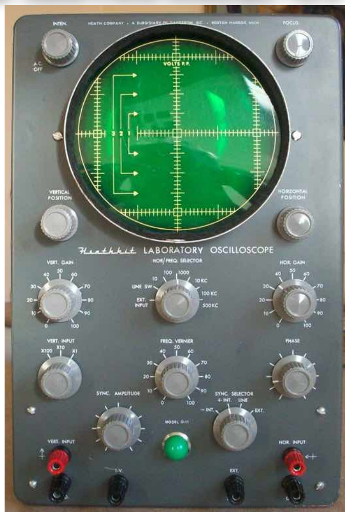
Figure 7: Heathkit O-11 Oscilloscope. Except for the pilot lens and model # the front panel is identical to the O-10. Photo by Keith Greenhalgh.
